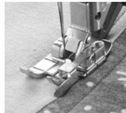
**Open-Toe Presser Foot** – Open-Toe Feet are made for decorative stitching and applique – the base of the foot has a groove in them to ride over the stitches getting thicker. Most thing that would be stitched with this foot – will probably need a stabilizer like tear away. Open-toe feet are not made for general sewing – with no material in the toe and the groove on the bottom – the fabric will get a lot of bounce and will prevent the machine from forming a good stitch.
