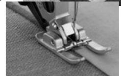
**Adjustable Bias Tape Foot**- This foot is available for most every machine on the market. It allows you to adjust to most any basic size of bias (or straight of the grain) bindings that you can buy pre-made or make yourself \*\*\*see bias tape makers & sashers in the next section. You can bind a quilt this way – however most quilters use a French Binding technique that allows for fabric along the edge and will last longer. This is great for craft items and clothing.
